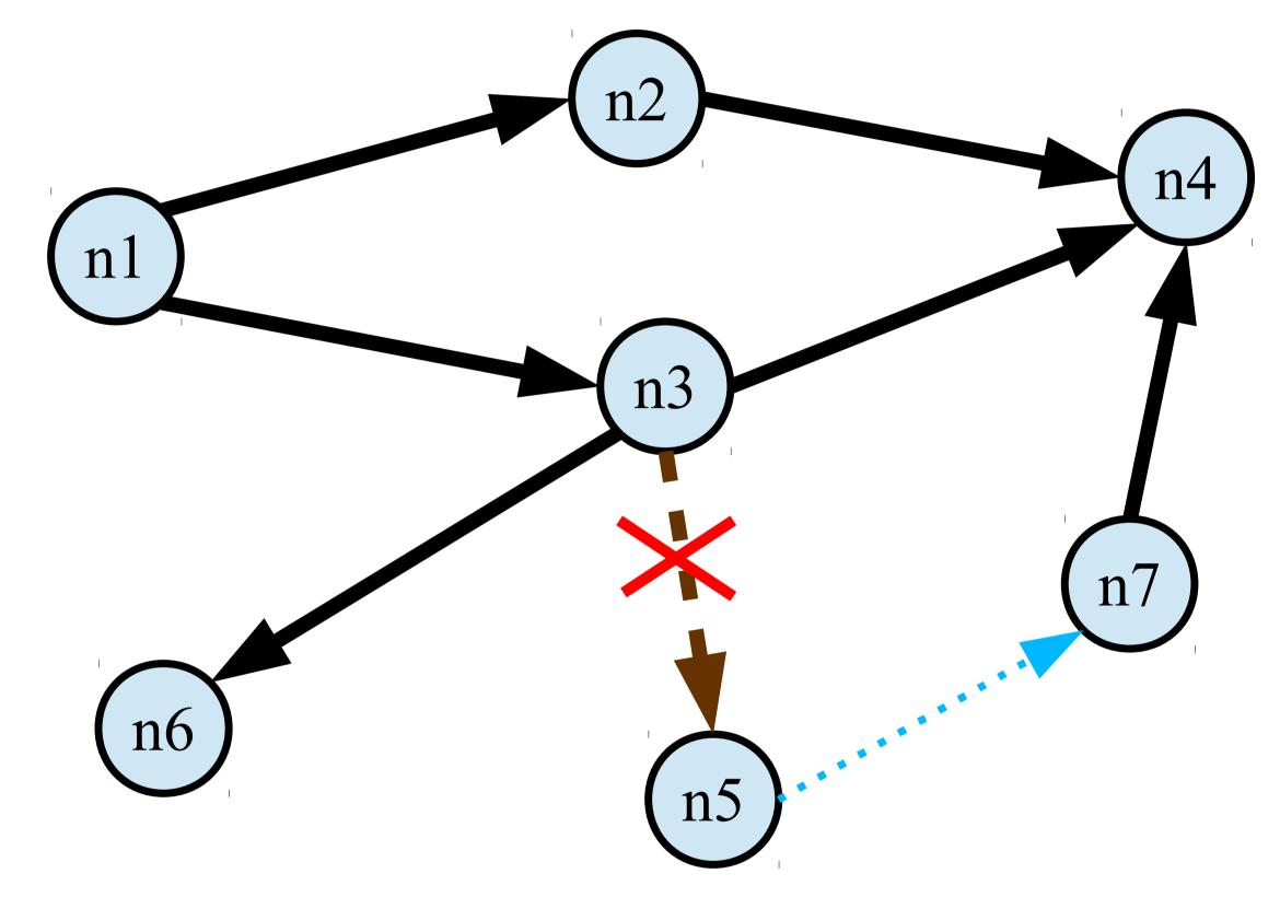
A graph undergoing an update which creates link (n<sub>5</sub>, n<sub>7</sub>) and an update which deletes (n<sub>3</sub>, n<sub>5</sub>), interleaved by a concurrent traversal query starting at host  $n_1$ . In absence of strong guarantees, the query can return path (n<sub>1</sub>, n<sub>3</sub>, n<sub>5</sub>, n<sub>7</sub>) which never existed at any instant.
